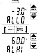
Reading ALLO indicates adjusted lower alarm limit (here air temperature). Set the desired value by means of the arrow keys. Press and hold the arrow key UP to make value increase fast. Press and hold the arrow key DOWN to make value decrease fast. Release the arrow key and press ENTER to confirm new limit.
